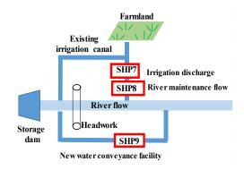
Figure 3 Mechanism of SHP in headwork
