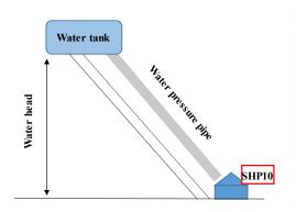
Figure 4 Mechanism of SHP in waterway
